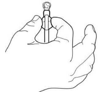
Figure 3: Actuation of Valve to Drain Bladder
